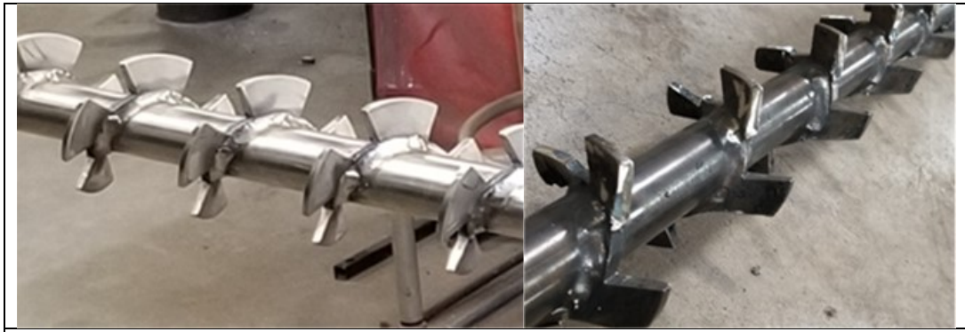
Figure 7.1. Shaft before (left) and after (right) modifications.
